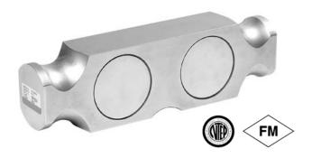
A reliable sealing and mechanical protection of the strain gage area is ensured by the use of potting compound with a metal cover.
